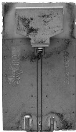
Fig. 4.3: Prototype of the Skycross SMT-3TO10M antenna. This antenna was used in all MCI and MCII measurements.
